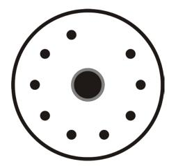
Do not insert preamp tubes with missing or damaged pins.
