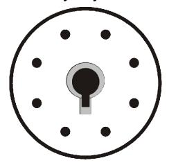
Do not insert power tubes with missing or damaged keys or pins.
