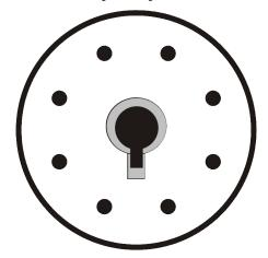
Do not insert power tubes with missing or damaged keys or pins.
